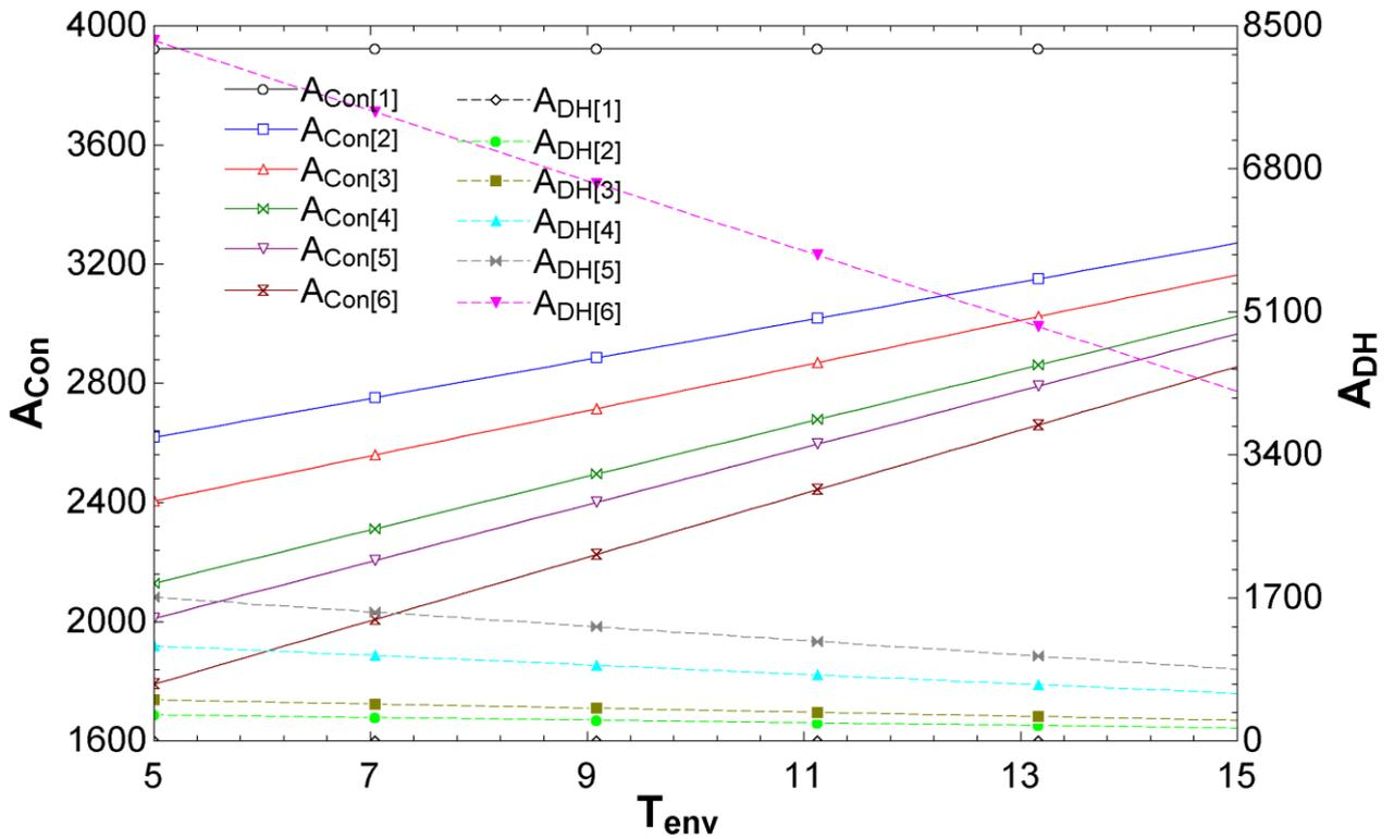
Fig. 8. Condenser and DH heat exchanger area with respect to the environmental temperature.
