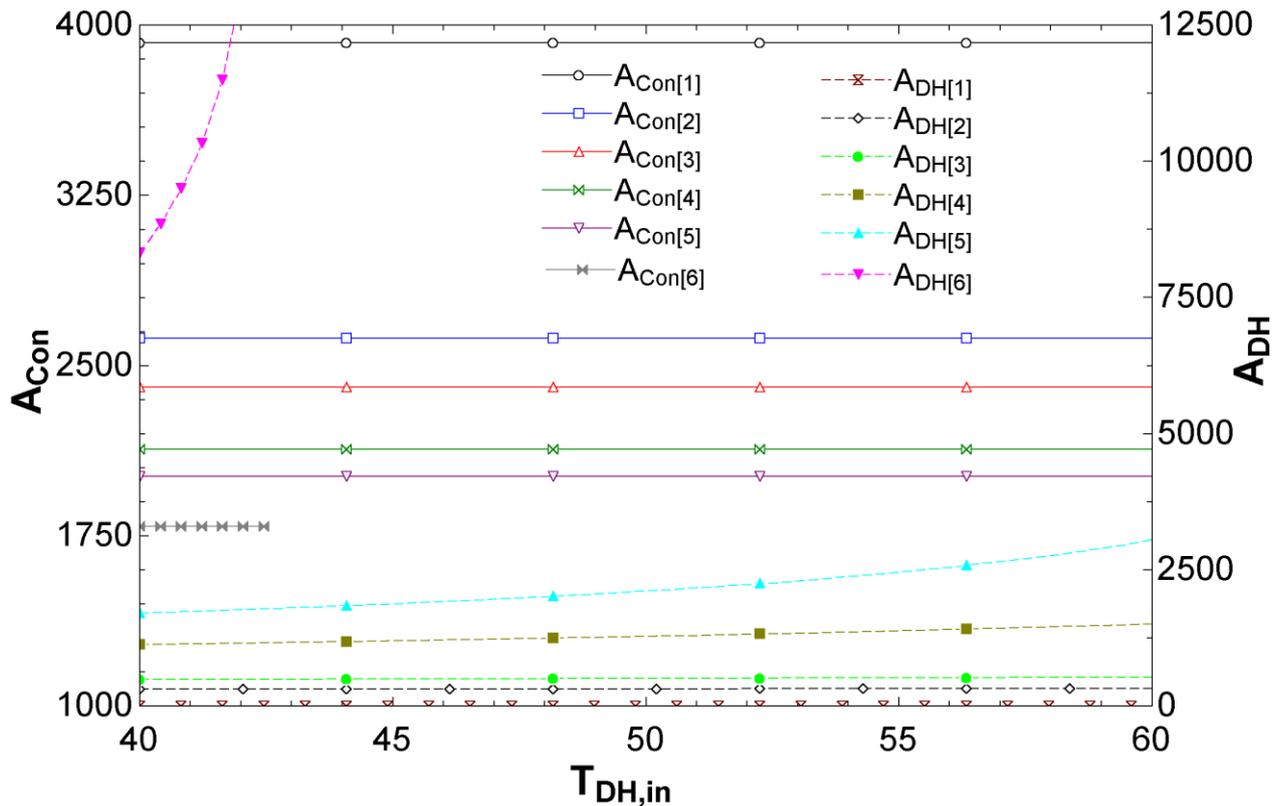
Fig. 9. Condenser and DH heat exchanger area with respect to the DH inlet temperature.
