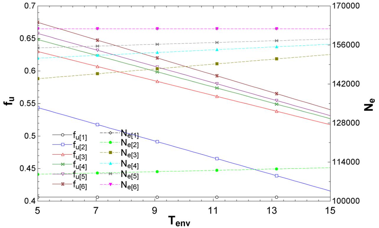
Fig. 6. Utilization factor and electricity loads with respect to the environmental temperature.
