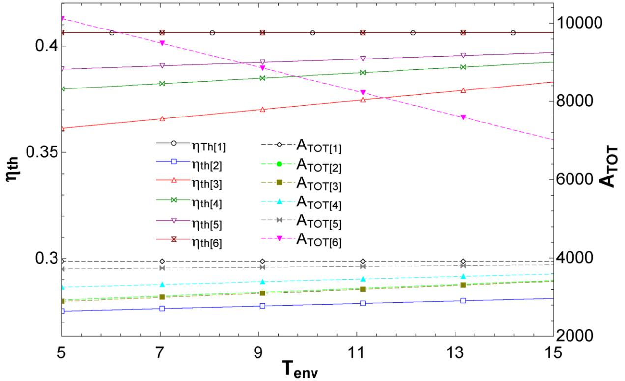
Fig. 7. Thermal efficiency and total heat exchanger area with respect to the environmental temperature.
