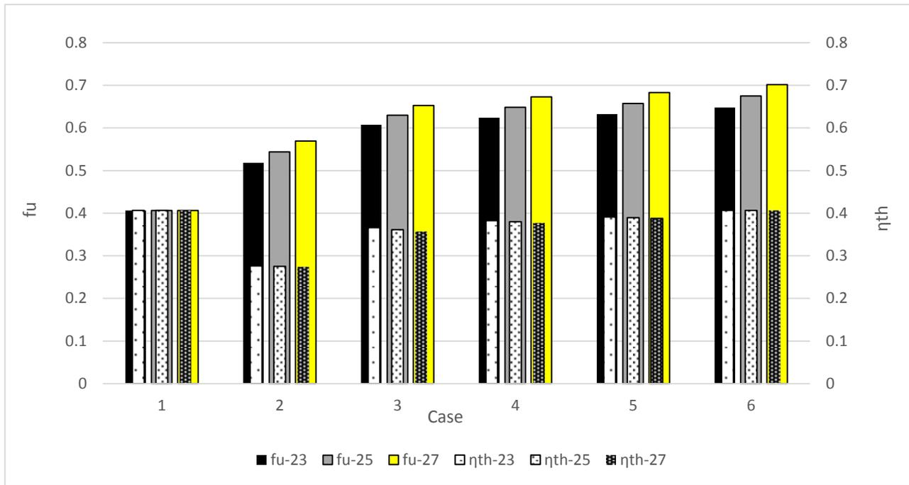
Fig. 4. Utilization factor and thermal efficiency with respect to the cases and inside comfort temperature.
