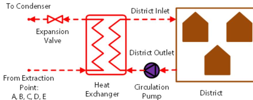
Fig. 2. Simplified general schematic of district heating system
